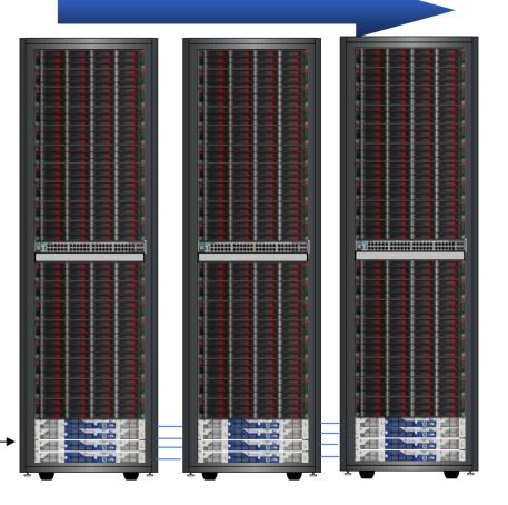
InfiniBand links across racks for full connectivity
