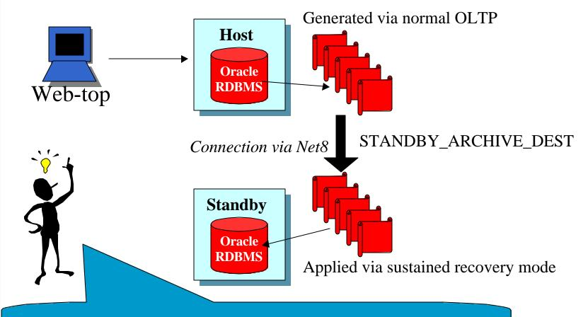
The standby is ready for use when production fails.
